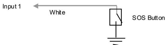
**Note:** input voltage to Input must not over 45V
